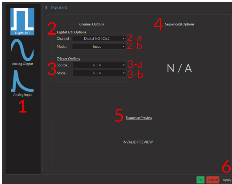
Figure 3.16: Channel(s) configuration window, Digital I/O input
