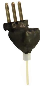
Fiber-optic Cannula + Single LED
