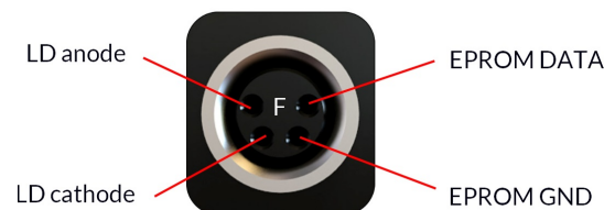
Laser Diode Module Driver female pinout
