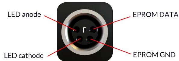
LED Driver female pinout
