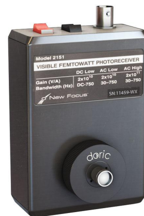
Newport Visible Femtowatt Photoreceiver Model 2151 + Doric FC Adapter
